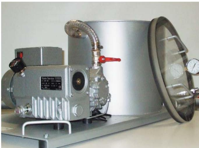
Compact, silent pumps, supplied complete with special synthetic oil and, unless otherwise requests, 5-metre cord with plug.
